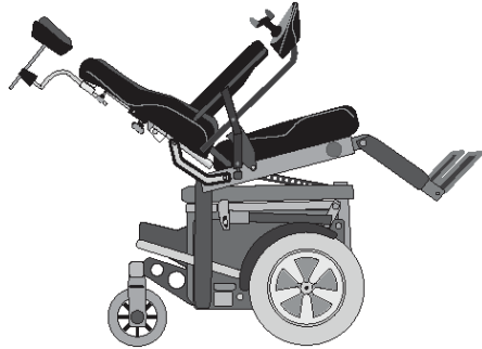
Figure 2. Front-wheel drive power wheelchair with recline capability.
